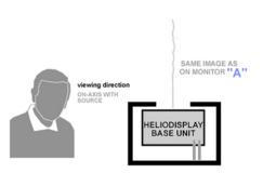
what you need: location, location, location (lighting,wind, etc) design adequate content (high contrast) plug in power cables plug in video cable charge base unit w/ 1L of regular tap water turn on system
